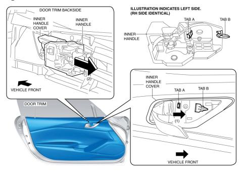
8. Remove the inner handle in the direction of the arrow (2) shown in the figure while detaching tab B.
