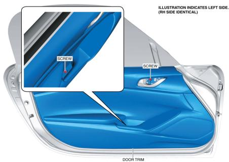
5. Move the door trim in the order of arrows (1), (2), (3), (4),(5) and (6) shown in the figure and detach the clips.
