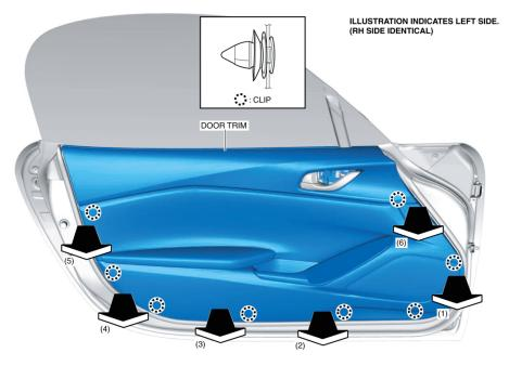
6. Remove the door trim in the direction of the arrow shown in the figure.
